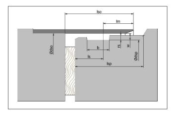
• Concrete jacking pipes must comply with the requirements of DIN EN 1916 and DIN V 1201.
