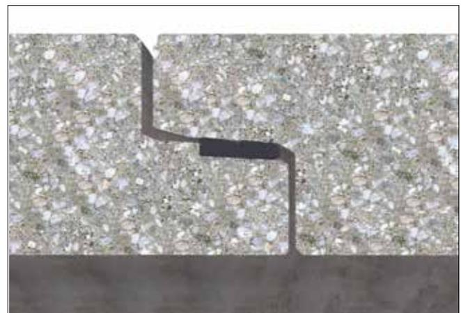
DS LK2L pipe connections can be installed without any problems using normal construction site equipment. When laying the pipes observe DIN EN 1610 and work sheet DWA-A 139.
