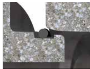
DS round ring M as pressure pipe seal
